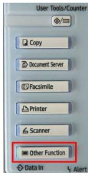
Figure 1: The Other Function key on an MFD with SDK 7.
